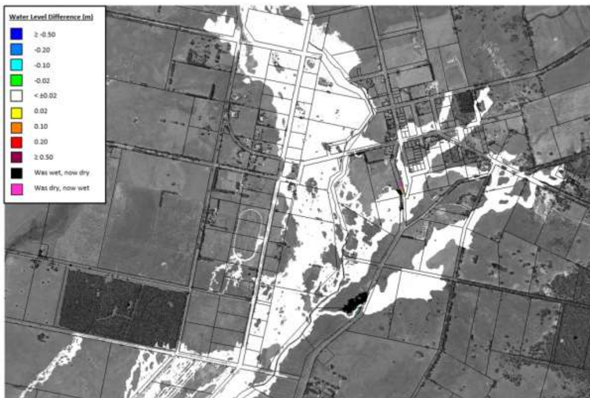
Plate 5 1% AEP change in flood levels due to raising Eurambeen - Raglan Road
