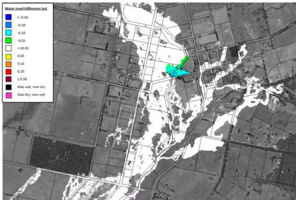
Plate 7 1% AEP change in flood levels due to widening the Fiery Ck crossing at Raglan - Elmhurst Rd
