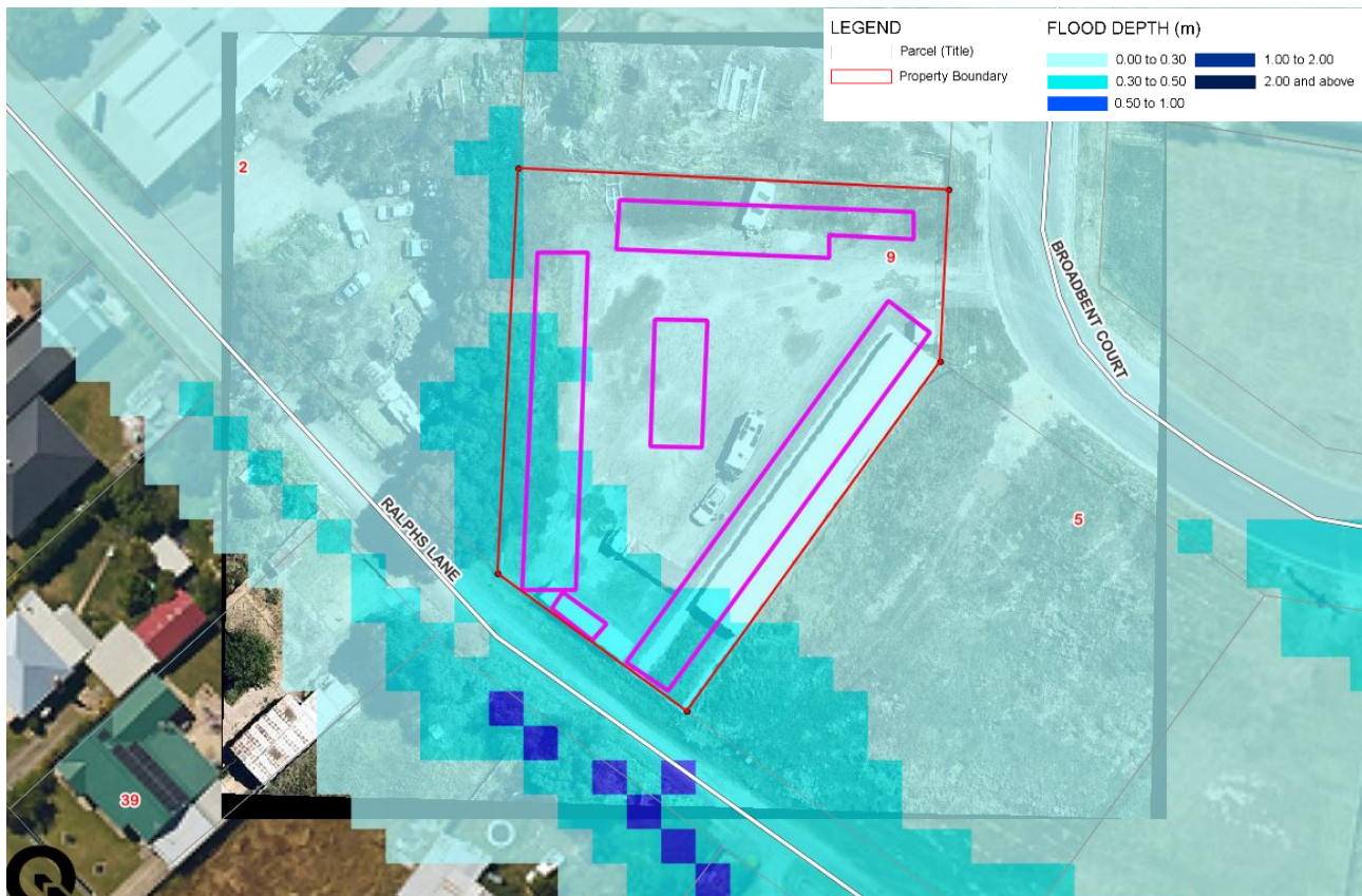
Figure 1. Showing estimated 1%AEP flood extent and depth with proposed shipping container positions (pink boxes) overlaying existing site including the existing shipping container row.
