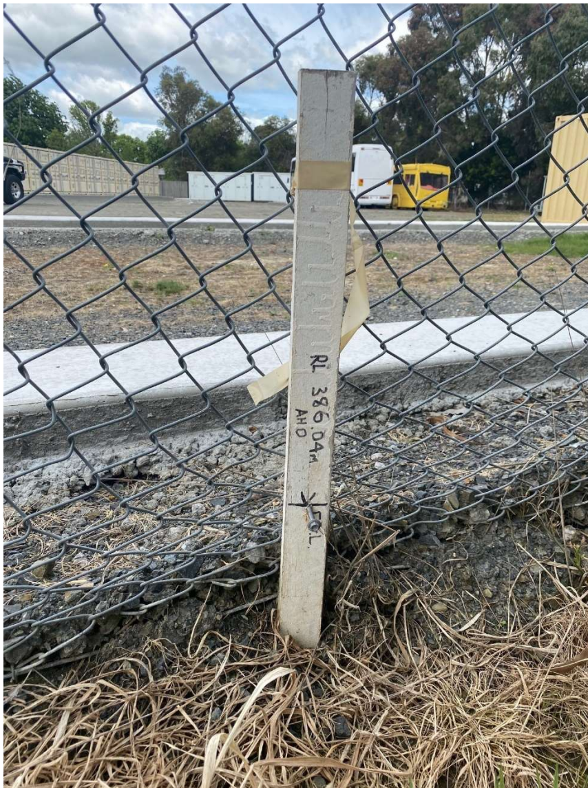
AHD Temporary benchmark on North Title Boundary F.F.L Noted for neighbouring development.
