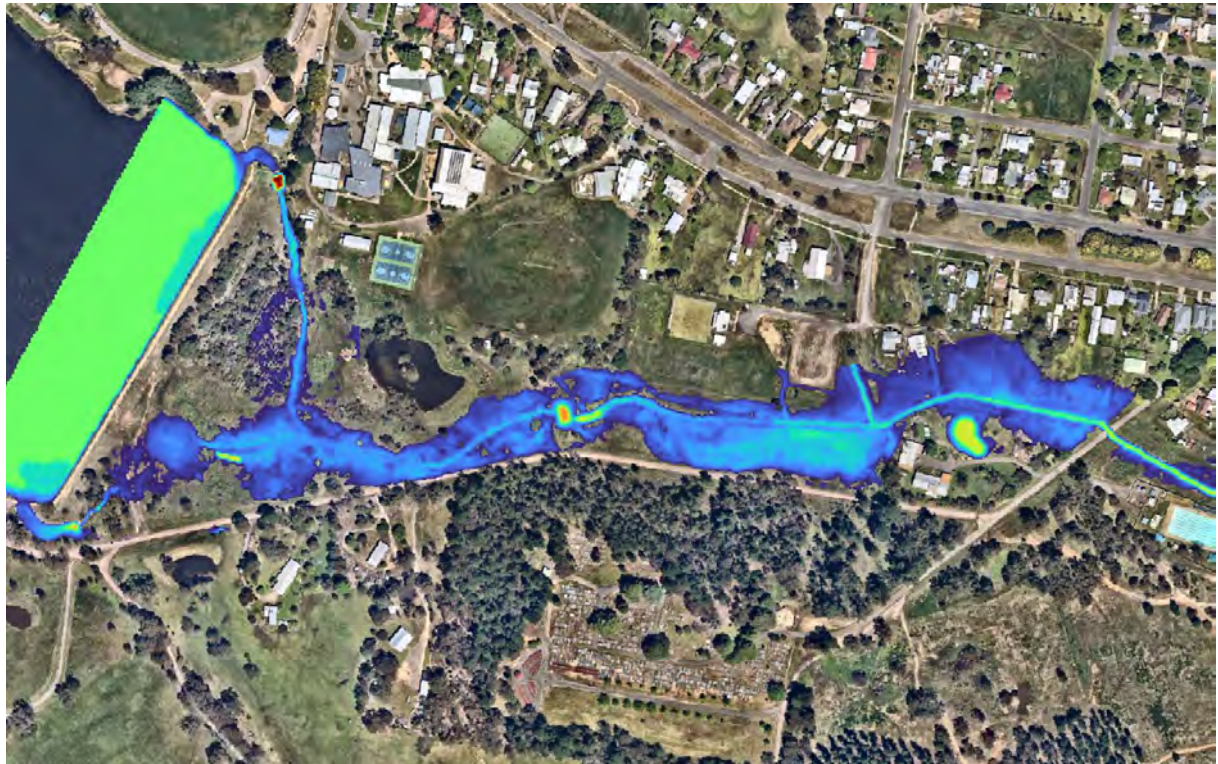
Plate 14: Scenario 3 – Flooding extent in the 1EY upstream of Havelock Street based on increase culvert size at Leichardt Street, underneath the central POS and conveyance channel
