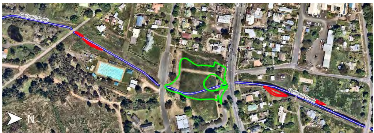
Plate 10: Proposed modifications to the Garibaldi Creek (i.e. changes to alignment in red and changes to topography in the central POS in green)
