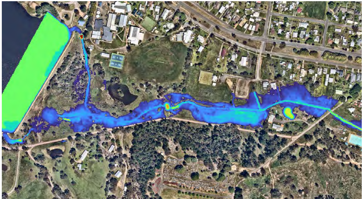
Plate 11: Scenario 2 – Flooding extent in the 1EY upstream of Havelock Street based on proposed changes to alignment and linear park within central POS
