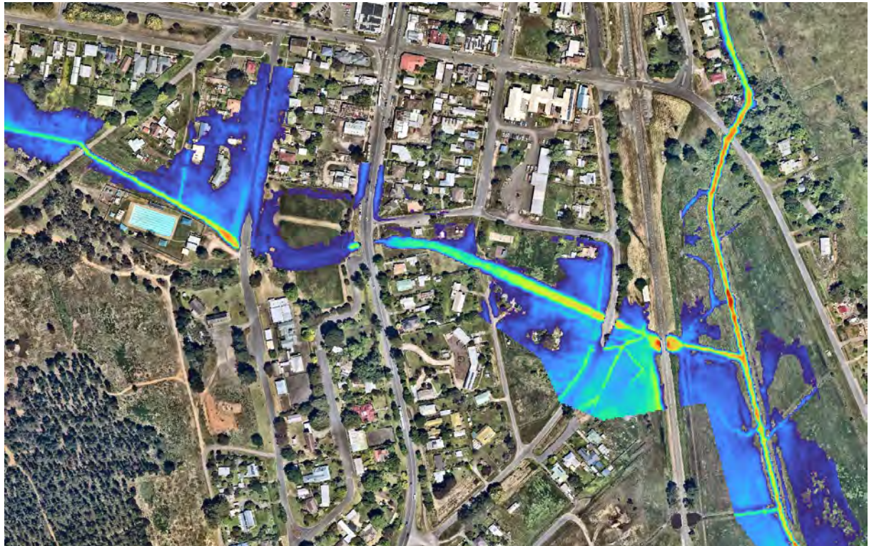
Plate 9: Scenario 1 – Existing flooding extent in the frequent rainfall event (1EY) downstream of Havelock Street
